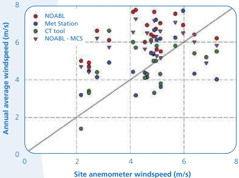
**Figure 4** Comparison of wind speed prediction models with anemometer measured wind speed data at fully monitored free standing pole mounted turbine sites. Met Station (measured), NOABL (predicted), MCS adjusted NOABL (predicted),
